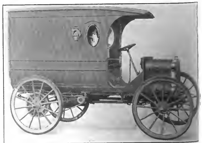
Fig. 3—Delivery Wagon type showing full elliptic rear spring suspension, large diameter wheels, and solid tires
